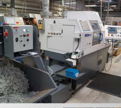
up to three times each week, often with large volumes of neat oil. Sean Keet says: "Now we only have to refill the sumps once a week and as the Oil Saver reclaims the coolant back from the swarf bin in to the same sump there is no chance of cross-contamination. This amounts to a significant amount of time saved across all the sliding head lathes.'
